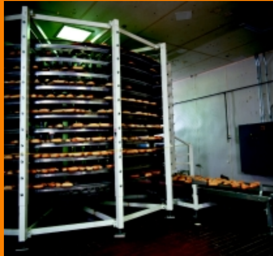
▼ Three ambient spiral cooling systems prepare baked foods for freezing.
